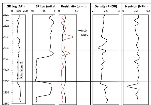
Fig.2: Composite log responses of the hydrocarbon bearing Zone 2 (2337-2350 m) identified in Mio-Pliocene sandstones of the well Rashidpur-4, Bangladesh [25].
